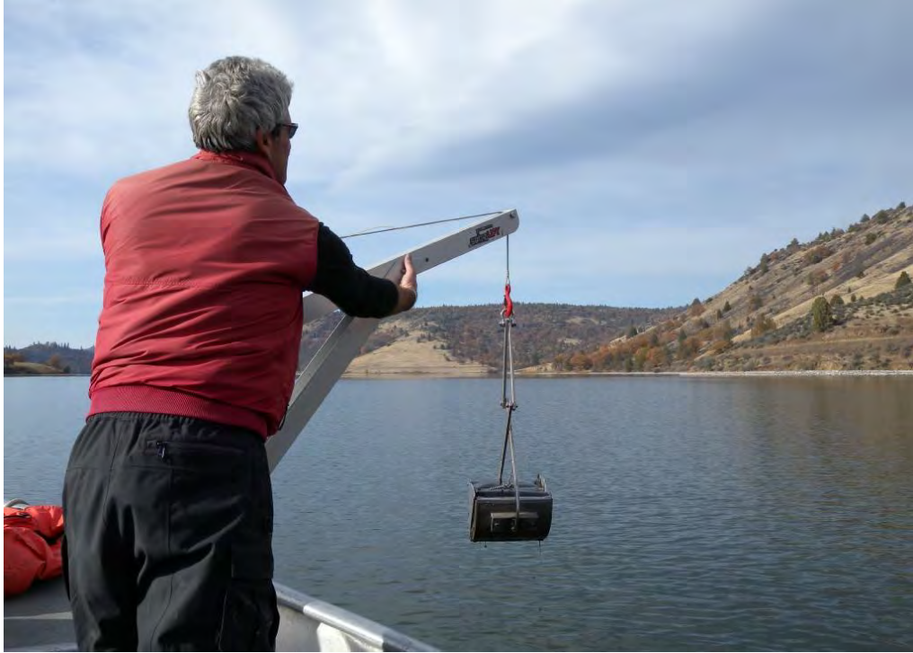
Figure 5-39. Ponar sampling device used to collected disturbed samples.
