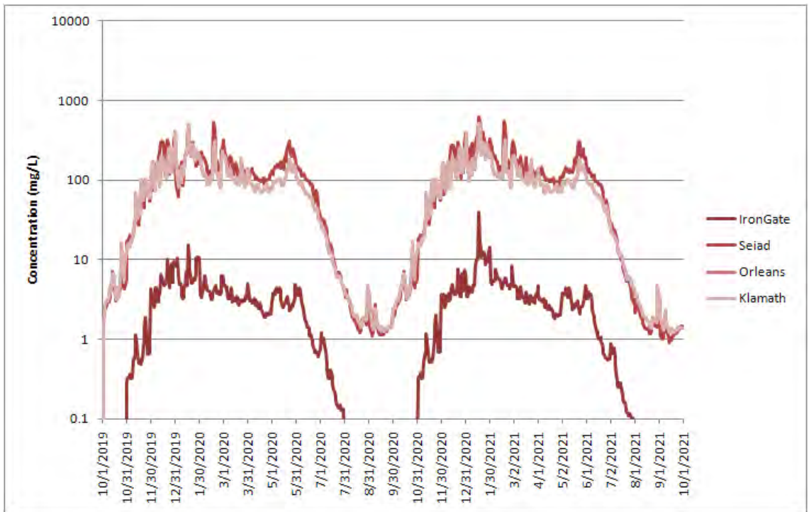
Figure 23-54. Sediment Concentrations at stream gage locations for background conditions at 10% exceedance levels.
