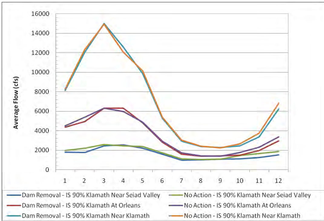
Figure 6-16. 90% Exceedance flows near Seiad Valley, Orleans, and Klamath for Dam Removal and No Action Alternatives.
