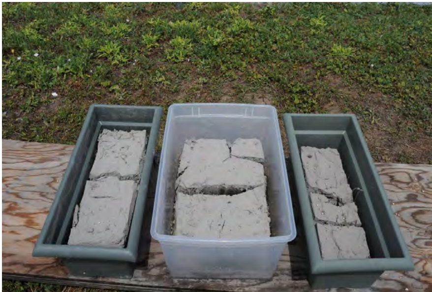
Figure 5-43. Picture of sediment from J.C. Boyle Reservoir 15 days after placement.
