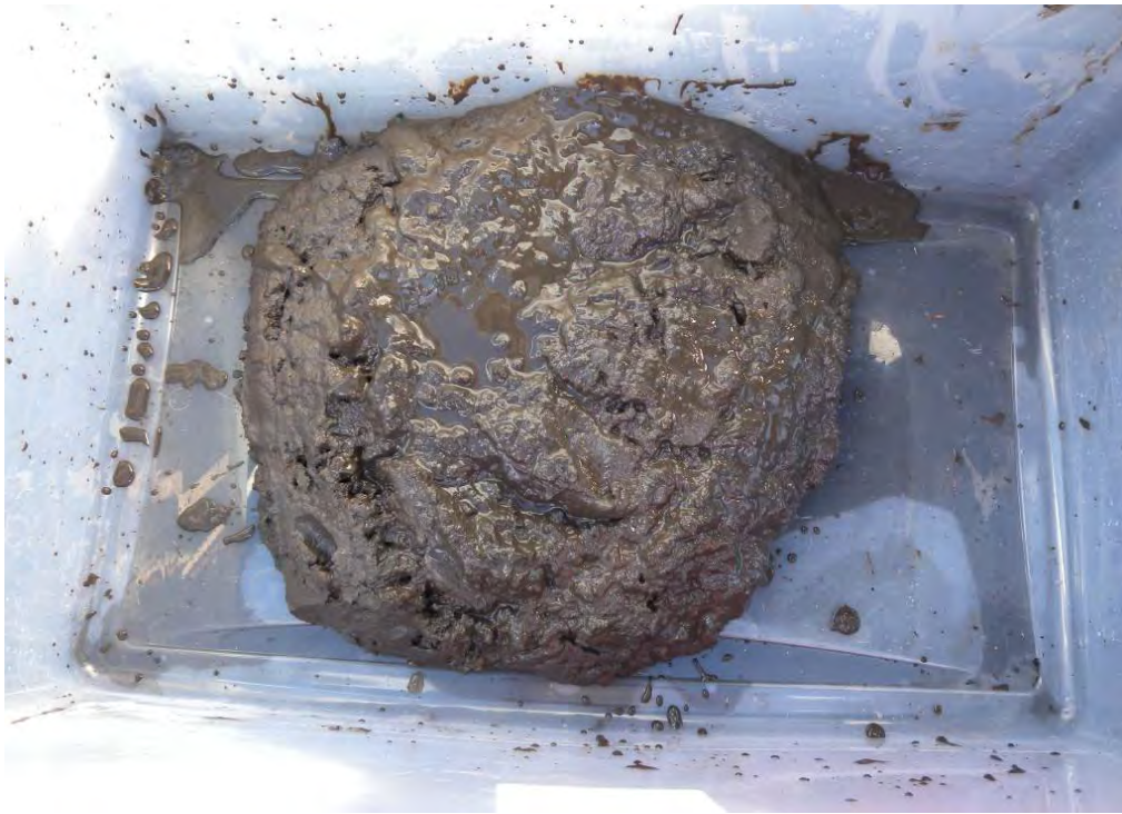
Figure 5-38. Sample just after release from Ponar sampling device.
